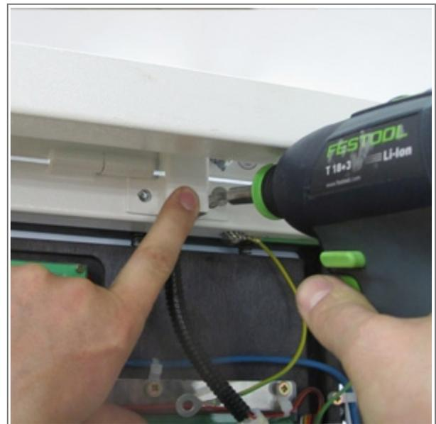
10. Remove a central barrier from the basketball and assemble it (2 screw M8x20). Connect a lighting system and speakers ||
