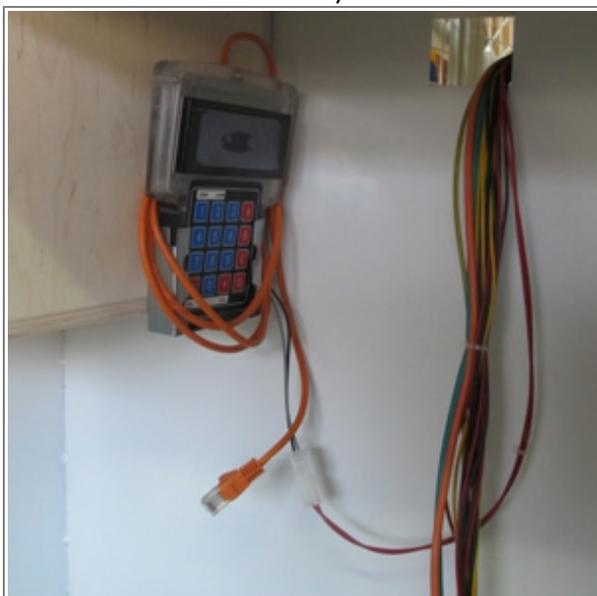
Now you can move to the option you want to set (e.g. 01, 05, 17) by pressing **B** (up) and **C** (down) buttons. To enter and change the option press **#** until the lower line with the position you want to change starts blinking.
